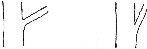
Wide crotches (left) are stronger than weak, narrow crotches (right).
